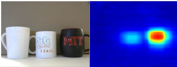
Fig. 5. Image from the in-hand palm camera and the corresponding thermal camera. The left cup is filled with water at room temperature, middle cup with warm water at 50°C and right cup with boiling water at 90°C
